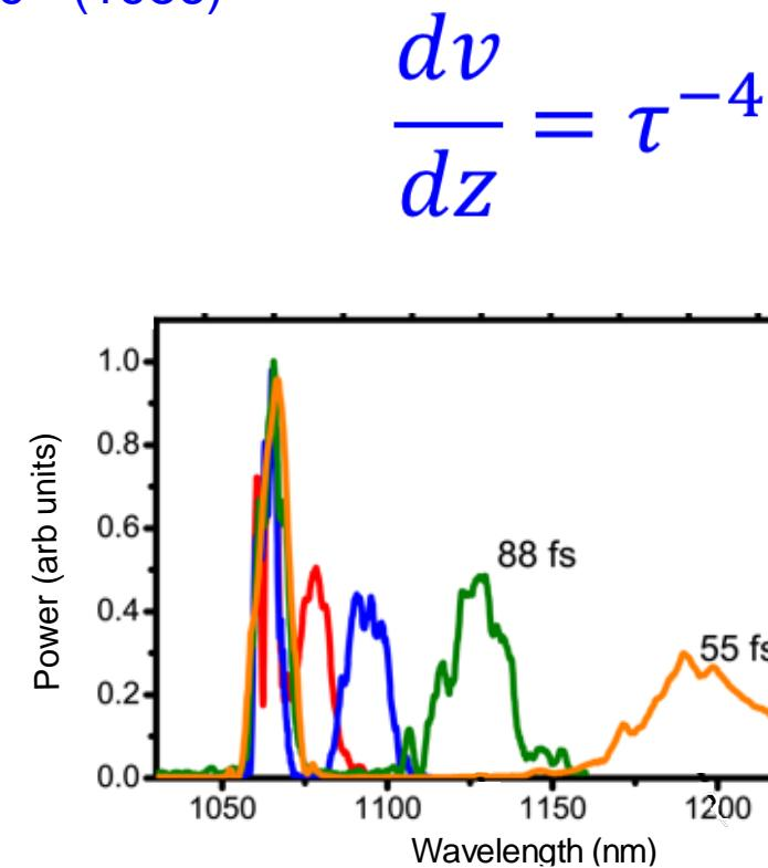
Raman gain pumped by cw Raman fibre laser
