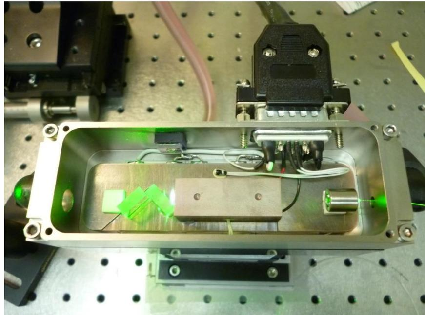
Frequency doubled, cw-seeded Raman fibre amplifiers for wavelength, pulsedwidth and repetition rate selectivity
