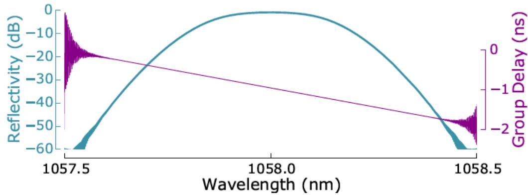
$$n_0 = 1.45 \quad \delta n = 5 \times 10^{-5} \quad L = 200\text{mm}$$
