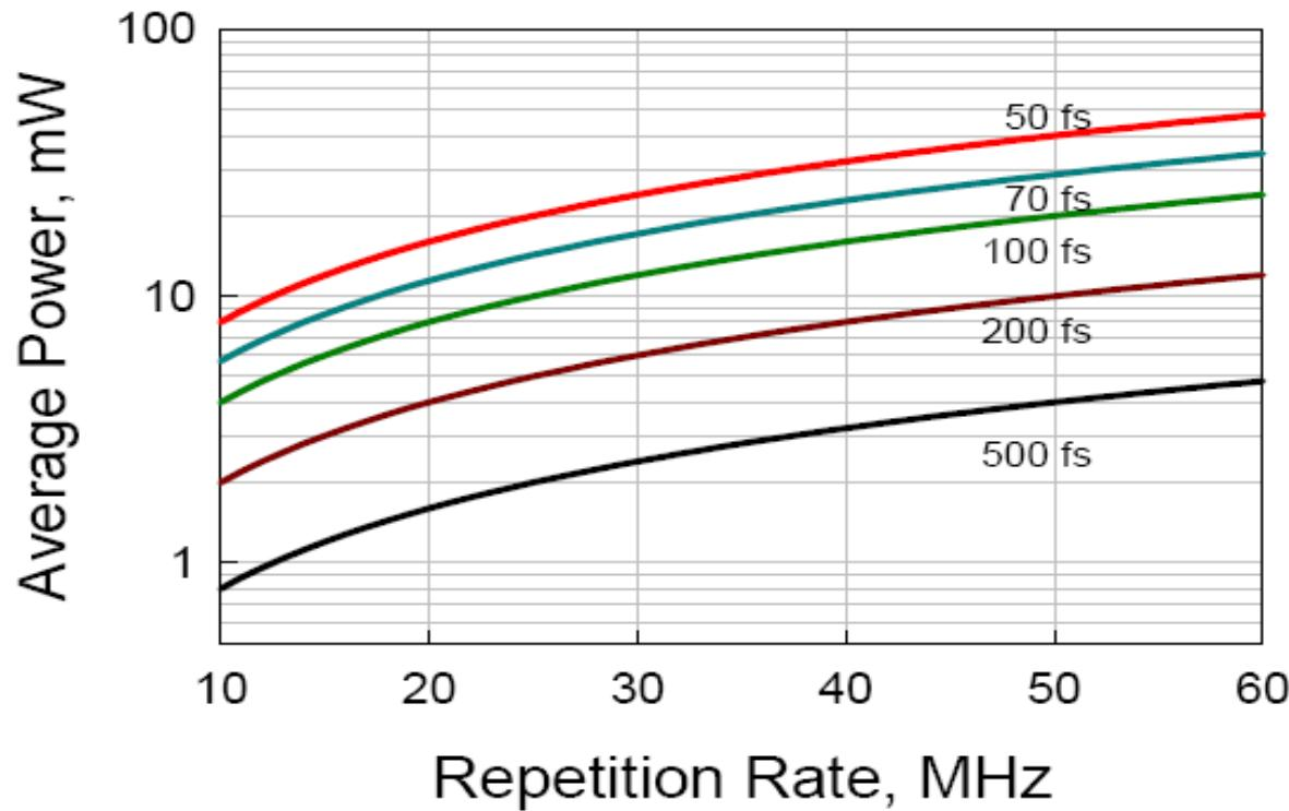
At repetition rates from a conventional fibre laser, for pulse durations in the 500fs-1ps regime only a few mw average power is required
