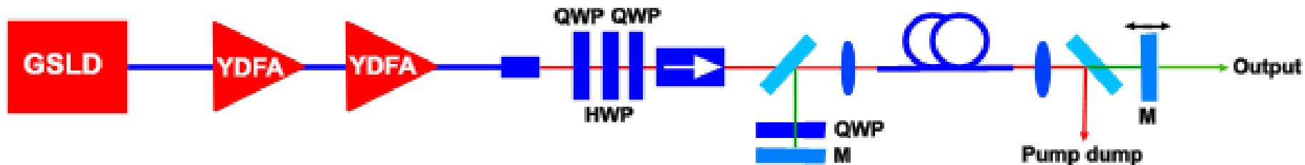
Pump - gain switched DFB at  $\sim 20$  MHz (17.984MHz) Amplified  $\sim 14$ W (3.5kW peak)
