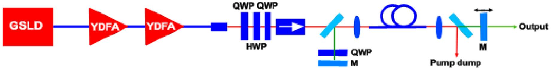
Pump - gain switched DFB at ~ 20 MHz (17.984MHz) Amplified ~ 14W (3.5kW peak)
