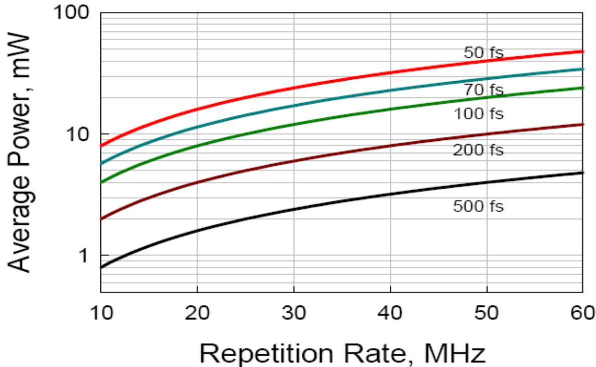
At repetition rates from a conventional fibre laser, for pulse durations in the 500fs-1ps regime only a few mw average power is required
