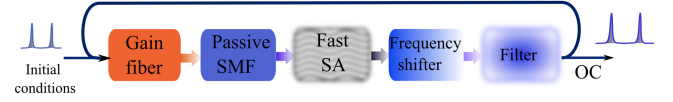
Fig. 3. The scheme of a fiber ring laser used in the numerical simulation. SA – saturable absorber, OC – output coupler, SMF – single-mode fiber.
